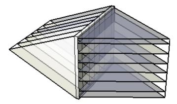
**Fig. 2.** A sketch of the Lenslet device used for performing vector-matrix multiplications. A vector of lasers (left part of the picture) generates the light which passes through a modulator and then is collected by an array of detectors (right part of the picture).
