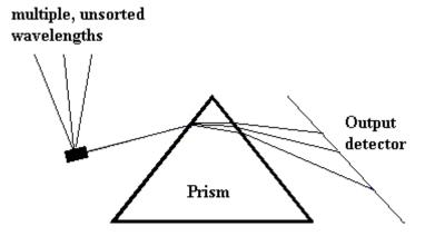
Fig. 3. Schematic view of the Rainbow Sort.
